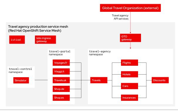
Figure 3. Travel by Keyboard's target service mesh architecture with connections to GTOs travel portal via APIs
