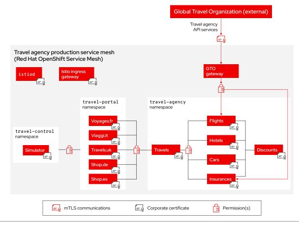
Figure 7. Final authentication and authorization configuration for the travel agency service mesh
