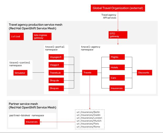
Figure 8. Travel agency service mesh architecture with connections to an external insurance broker partner system
