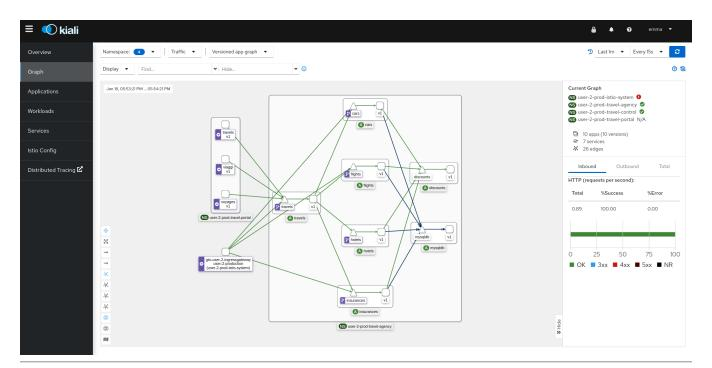
Figure 4. Kiali visualization of the new Istio configuration
